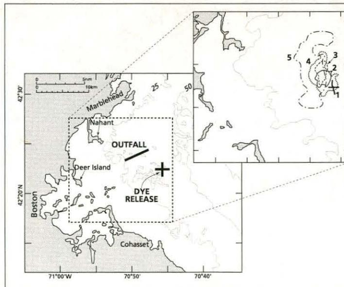
Rhodamine dye was released into Massachusetts Bay in the shape of a '+' in August, 1993. The vertical and horizontal spreading of the dye was monitored for the next 4 days. Horizontal spreading of the dye is depicted in the inset (numbers correspond to days, 1 being the deployment day). The spreading of the dye patch allows the mixing rates of the Bay to be quantified, which will lead to more accurate estimates of the dilution and transport of the sewage effluent.
