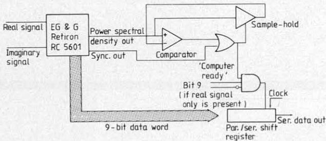
Figure 1. Block diagram of the circuit for determining the frequency of peak spectral amplitude.
