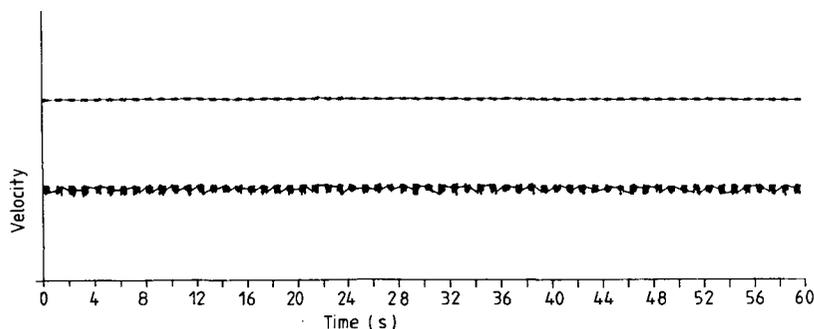
**Figure 4.** FFT-tracker comparison when input frequency is held constant and SNR = 0 dB.
