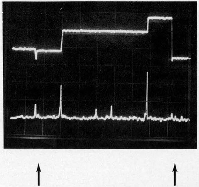
Figure 2. The Fourier spectrum of an incoming signal (lower trace), and the peak position detecting sample-hold output (upper trace). The full 512-point spectrum is displayed between arrows. The second strongest peak is the reflected frequency,  $\omega$ . In our set-up with real signals, only the first half spectrum is used. The small peak at left arrow is the DC spectral threshold. (The same threshold at the right arrow appears diminished due to aliasing of the digital oscilloscope used.)
