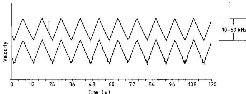
**Figure 3.** A comparison of the FFT processor described here (upper trace) and the DISA 55N20 tracker (lower trace).
