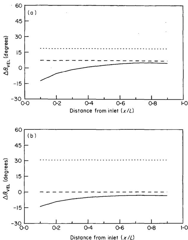
Figure 3. Comparisons of the tidal velocity phase differences for the numerical solution (—), the nonlinear continuity solution (---) and the linear solution (···) for (a) a v-shaped channel ( $b_0 = 0, \beta = 20$ ) and (b) a rectangular channel ( $b_0 = 50 \text{ m}, \beta = 0$ ) ( $h = 3.0 \text{ m}, L = 10 \text{ km}, f = 0.04, \text{Amp}_{M_2, \text{inlet}, \text{elev}} = 0.8 \cos(kL), \text{Amp}_{M_4, \text{inlet}, \text{elev}} = 0.0$ ).
