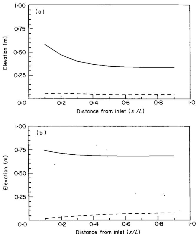
Figure 6. Numerical solution for the elevation amplitude of the fundamental (—), and harmonic frequencies (---) for (a) a *v*-shaped ( $b_0=0$ ,  $\beta=20$ ) and (b) a rectangular channel ( $b_0=50$  m,  $\beta=0$ ). Same parameters as given in caption to Figure 3.
