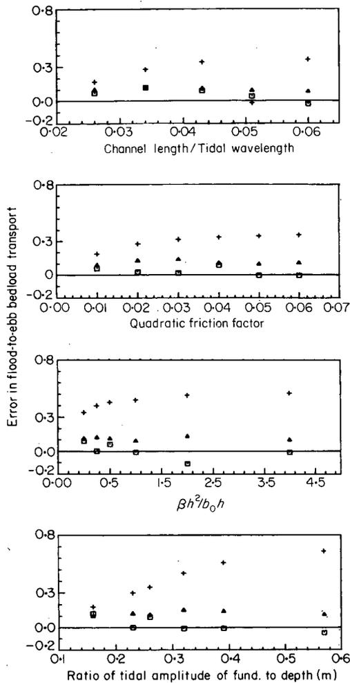
Figure 12. Error determination of the nonlinear continuity solution in terms of the ratio of flood-to-ebb bedload transport as a function of various parameters of the system and distance along channel [ $\square$ ,  $x/L=0.8$ ;  $\Delta$ ,  $x/L=0.5$ ;  $+$ ,  $x/L=0.2$ ]. ( $\text{Amp}_{M_1, \text{inlet, elev}} = 0.8 \cos(kL)$ ,  $\text{Amp}_{M_1, \text{inlet, elev}} = 0.0$ ,  $h = 3$  m,  $L = 10$  km,  $b = 50$  m,  $\beta = 0.0$ ,  $V_{\text{crit}} = 0.0$ ).
