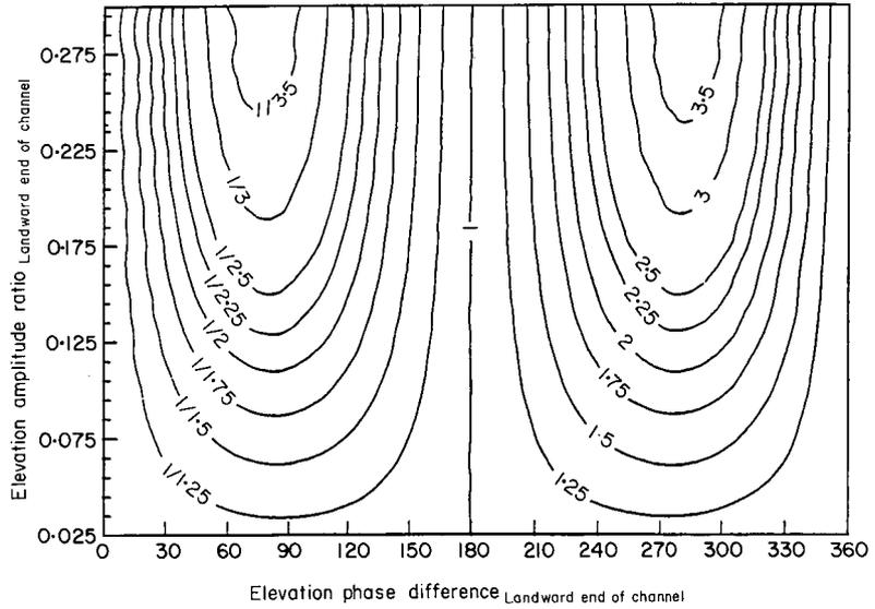
Figure 8. Tidal elevation asymmetry vs. flood-to-ebb ratio of bedload sediment transport. Velocity is nonlinearly related to elevation, critical velocity is zero and the relation holds for the length of channel if the channel length is much less than the wavelength of the tide ( $\eta_1/h = 0.3 V_{crit} = 0 \text{ cm s}^{-1}$ ).
