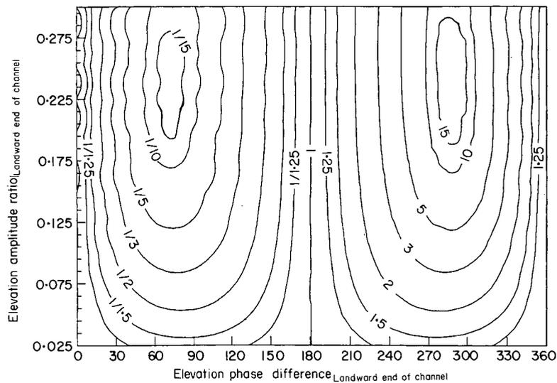
Figure 11. Tidal elevation asymmetry *vs.* flood-to-ebb ratio of bedload sediment transport 2 km from the inlet. Velocity is nonlinearly related to elevation,  $V_{crit} = 20 \text{ cm s}^{-1}$ ,  $L = 10 \text{ km}$ ,  $h = 3 \text{ m}$ .
