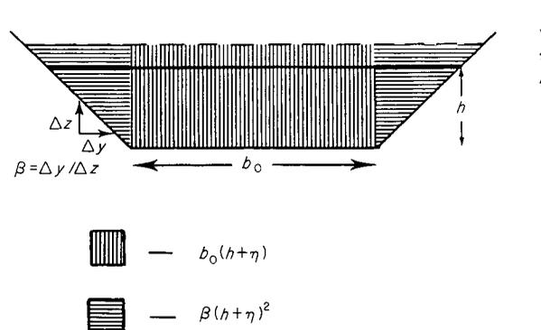
Figure 1. Channel geometry. The area of the channel that is marked by the vertical stippling is the area that changes in height only due to a change in tidal elevation. The horizontal stippling indicates the area of the channel that changes in both height and width due to a change in tidal elevation  $\beta(h+\eta)^2$ .
