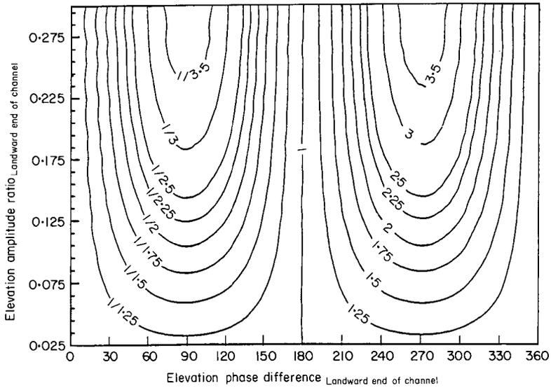
Figure 7. Tidal elevation asymmetry vs. flood-to-ebb ratio of bedload sediment transport. Velocity is linearly related to elevation, critical velocity is zero and the relation holds for the length of channel if the channel length is much less than the wavelength of the tide ( $V_{crit} = 0 \text{ cm s}^{-1}$ ).
