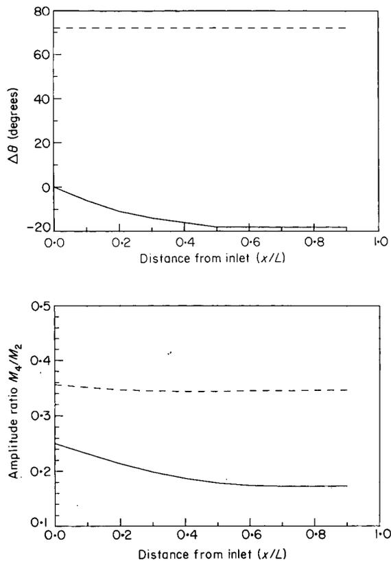
Figure 2. Comparisons between tidal elevation (—) and velocity (---) amplitude ratio and phase difference for a linear system with friction. ( $h = 3.0$  m,  $L = 10$  km,  $b_0 = 50$  m,  $\beta = 0$ ,  $\text{Amp}_{M_2, \text{inlet, elev}} = 0.8$ ,  $\text{Amp}_{M_v, \text{inlet, elev}} = 0.2$ ,  $\Delta\theta_{\text{inlet, elev}} = 0^\circ$ ).
