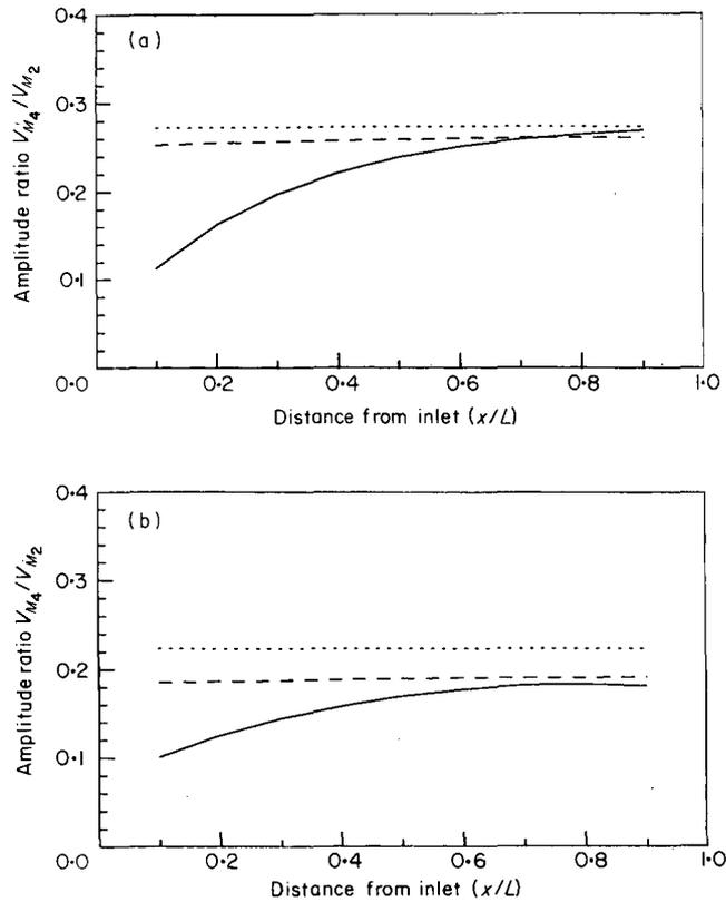
Figure 4. Comparisons of the tidal velocity amplitude ratio for the numerical solution (—), the nonlinear solution (---) and the linear solution (· · ·) for (a) a v-shaped channel ( $b_0=0, \beta=20$ ) and (b) a rectangular channel ( $b_0=50\text{ m}, \beta=0$ ). Same parameters as given in caption to Figure 3.
