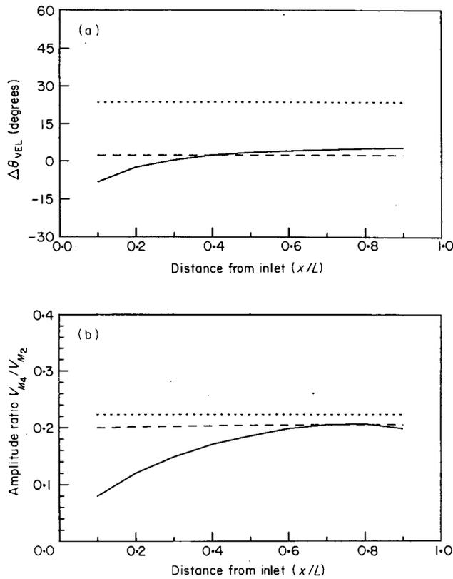
Figure 5. Comparisons of (a) the phase difference and (b) the amplitude ratio for velocity between the numerical solution (—), the nonlinear continuity solution (---) and the linear solution (···) for a channel with a flat bottom and sloping side walls. ( $h=3$  m,  $L=10$  km,  $f=0.04$ ,  $b_0=30$  m,  $\beta=10$ ,  $\text{Amp}_{M_2, \text{inlet, elev}}=0.8\cos(kL)$ ,  $\text{Amp}_{M_3, \text{inlet, elev}}=0.0$ ).
