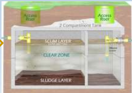
Existing Title 5 Septic Tank
