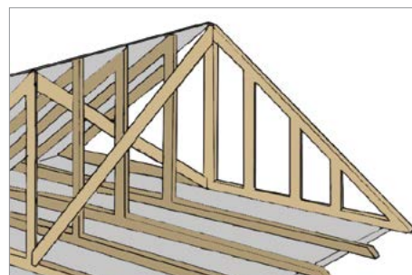
Figure 4-4. Diagonal braces form an X pattern from the top center of the gable end to the bottom center of the fourth truss and from the bottom center of the gable end to the top center of the fourth truss. The same screws as for lateral bracing are used. Source: FEMA's Against the Wind brochure 247.
