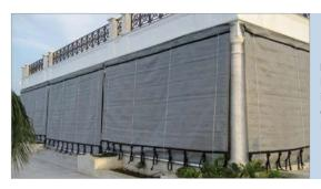
Figure 4-13. Polyethylene basketweave fabric windscreen is deployed at edge of patio, enclosing the entire area. Image courtesy of Roll-a-way.
