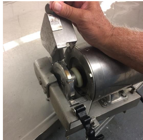
Oyster "shell breaker", the oyster is inserted bill end into the grinding surface making a simple entry point for the shucking knife
