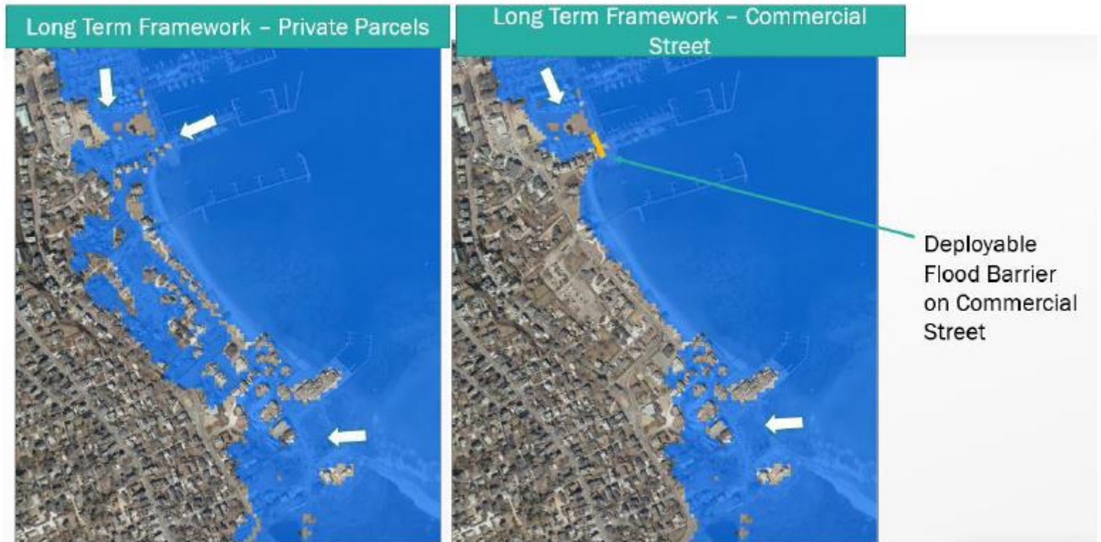
Figure 4: Flood extents during a 10% storm in Present Day, for existing (left panel) and with the proposed design (right panel) Alternate Grids
