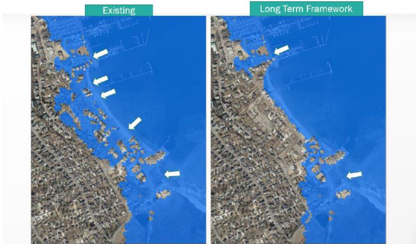
Figure 3: Flood extents during a 10% storm in Present Day, for existing (left panel) and with the proposed design (right panel)
