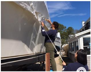
Cut the wrap above the strap at the belly of the boat, so the strap falls away, leaving only shrink wrap.
