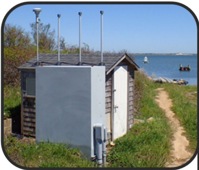
Air monitoring shed at Wampanoag Lab that houses the IMPROVE PM 2.5 samplers (left) Inside one of the 4 sampling modules where particulates are collected (right)
