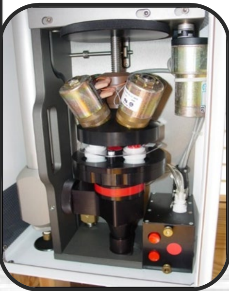
Air monitoring shed at Wampanoag Lab that houses the IMPROVE PM 2.5 samplers (left) Inside one of the 4 sampling modules where particulates are collected (right)
